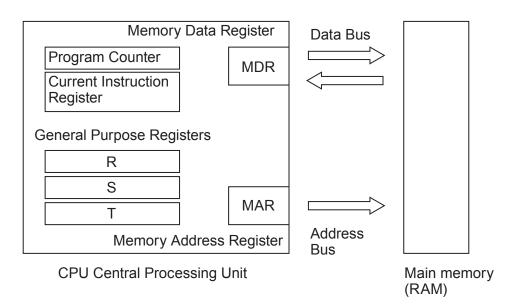
The computer has just completed a Fetch-Execute cycle in which a numerical value has been calculated and placed in a general purpose register R.
